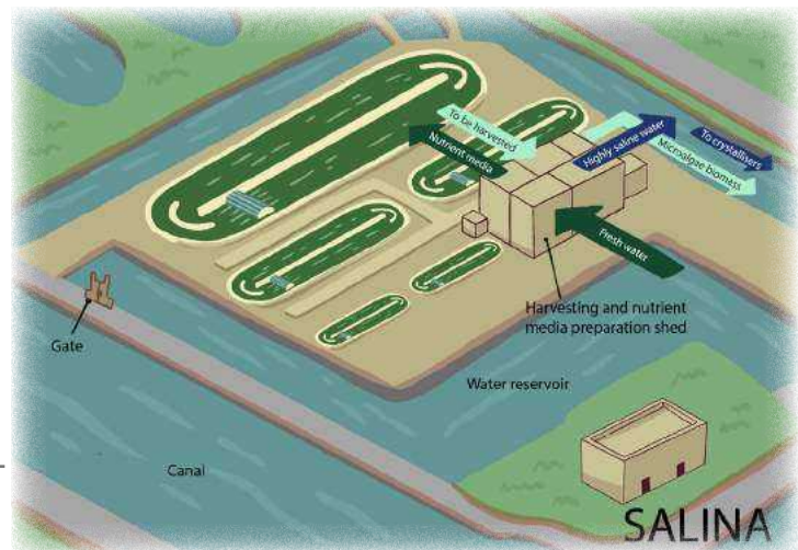
Figure 36. Design of an experimental microalgae plant in salina. ©PROARTE
