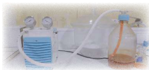
Figure 46. Device for D. salina carotenoids extraction by air bubbling at laboratory scale. ©SAIDA S.A.
