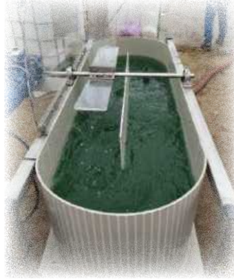
Figure 37. 200-litre capacity raceway-type reactor built within the framework of the MedArtSal subgrant programme at the Preciosa y Roqueta salina (Bay of Cadiz, Spain). It is made of polypropylene on a metal support so that its location can be changed. ©MedArtSal project
